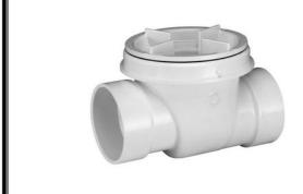
A backwater valve is typically a PVC plumbing fitting that is installed in the main sanitary sewer lateral at the end of the dwelling's drainage system and before connecting to the sanitary sewer main. They can be installed in the interior or exterior of the dwelling. Either location, they must have access to be cleaned and inspected.
