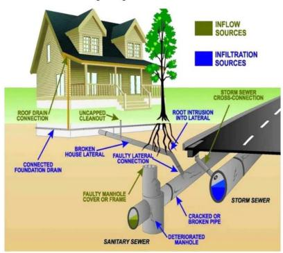
Reduce inflow and infiltration into the public sanitary sewer system.
