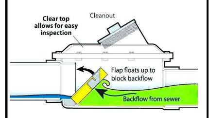
A backwater valve is a plumbing fitting that prevents the backward flow of sewage that might come from the sanitary sewer main following a blockage or surcharge. When sewage flows backwards, the flap in the backwater valve gets pushed by sewage and seals up the flow from coming back into the dwelling.
