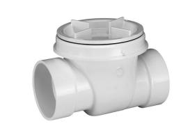
A backwater valve is typically a PVC plumbing fitting that is installed in the main sanitary sewer lateral at the end of the dwelling's drainage system and before connecting to the sanitary sewer main. They can be installed in the interior or exterior of the dwelling. Either location, they must have access to be cleaned and inspected.
